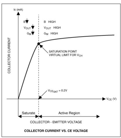
Figure 3. Bipolar signal transistors in the input stage must operate in the active region.
