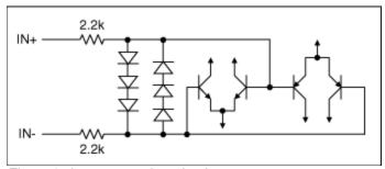
Figure 2. Input protection circuit.
