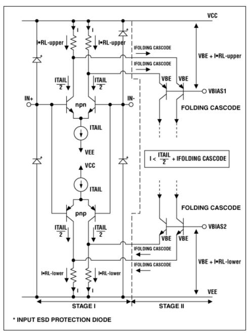
Figure 1. Maxim's Beyond-the-Rails input structure includes overvoltage protection.
