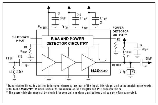
Figure 2. MAX2242 typical application circuit.
