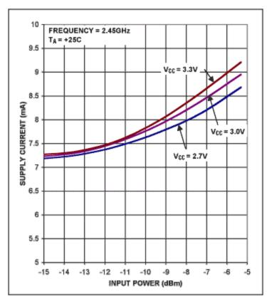
Figure 10. The MAX2644's supply current vs. input power.
