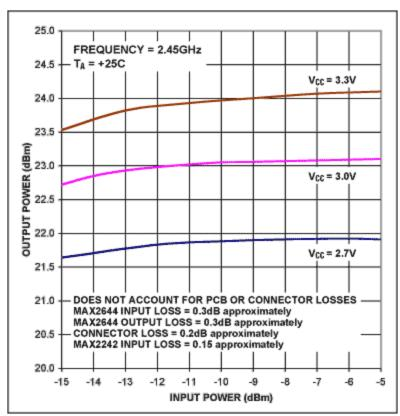
Figure 11. MAX2644 and MAX2242 cascaded performance.
