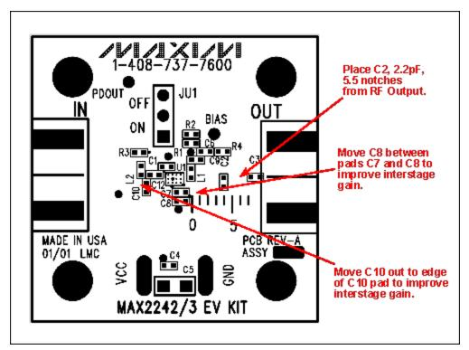
Figure 3. MAX2242 +23dBm component-placement guide.
