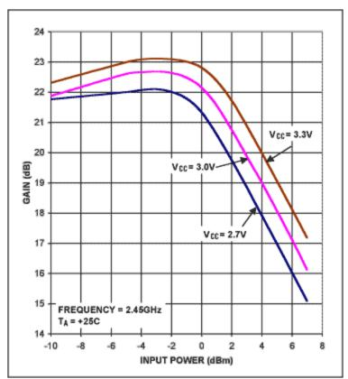
Figure 5. The MAX2242 PA's gain vs. input power.
