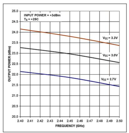
Figure 7. The MAX2242 PA's output power vs. frequency.
