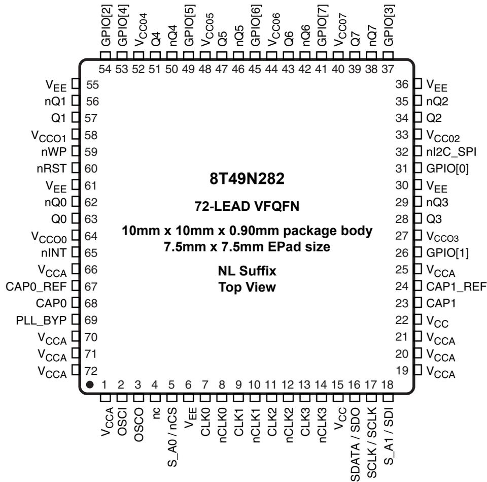
Figure 2. Pinout Drawing
