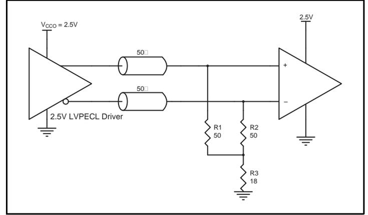
Figure 14C. 2.5V LVPECL Driver Termination Example
