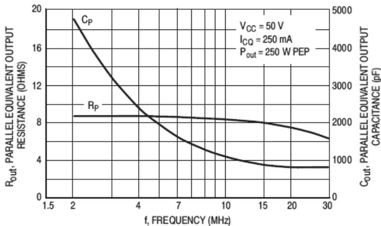
Figure 8. Output Resistance and Capacitance versus Frequency
