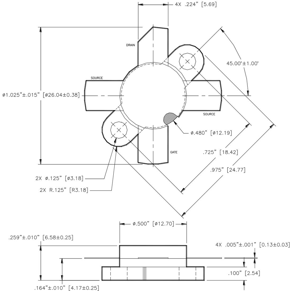
Unless otherwise noted, tolerances are inches  $\pm 0.005$  [millimeters  $\pm 0.13\text{mm}$ ]
