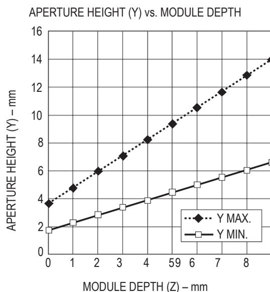
Figure 21. Aperture height (Y) vs. module depth.
