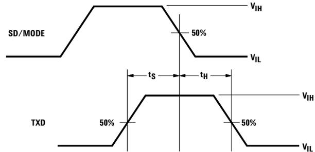
Figure 4. Bandwidth selection timing at FIR mode.
