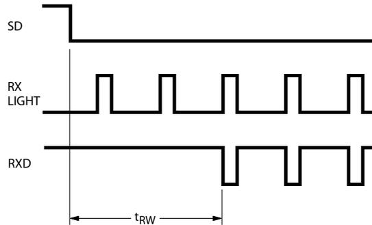
Figure 8. Receiver wakeup time waveform.
