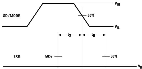
Figure 3. Bandwidth selection timing at SIR/MIR mode.
