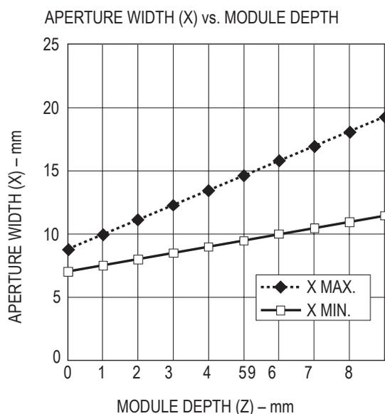
Figure 20. Aperture width (X) vs. module depth.
