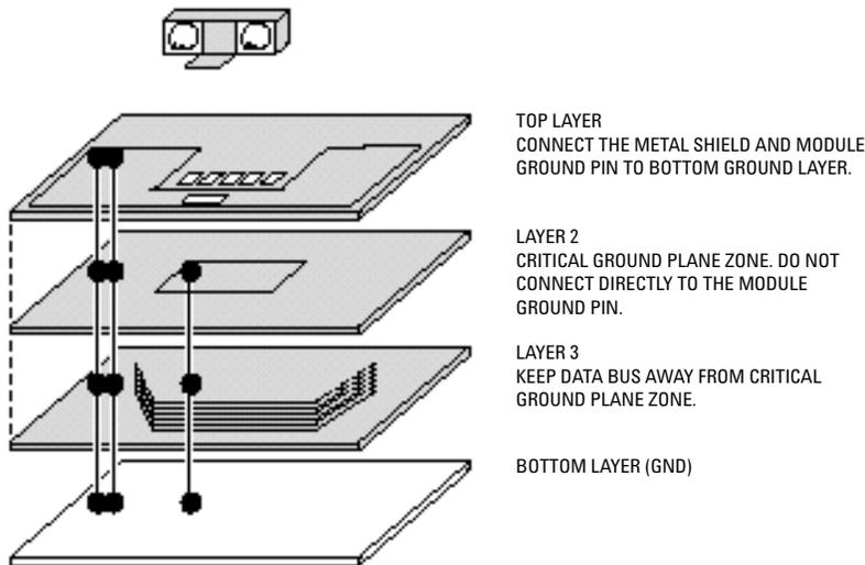
The area underneath the module at the second layer, and 3 cm in all directions around the module is defined as the critical ground plane zone. The ground plane should be maximized in this zone. Refer to application note AN1114 or the Lite-On Technologies' IrDA Data Link Design Guide for details. The layout below is based on a 2-layer PCB.
