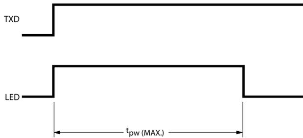
Figure 7. TxD "Stuck On" protection waveform.
