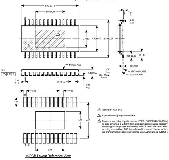
Figure 19: Package LP, 28-Pin TSSOP with Exposed Thermal Pad
