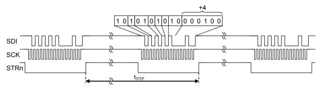
Figure 13: Serial Interface Sequence for Quarter Step in Forward Direction
