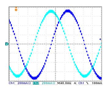
Figure A9: Measured Sixteenth-step Phase Current Sequence
