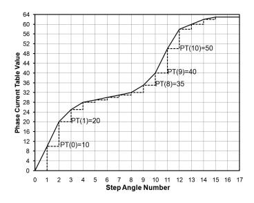
Figure 14: Digitizing the Example Current Profile
