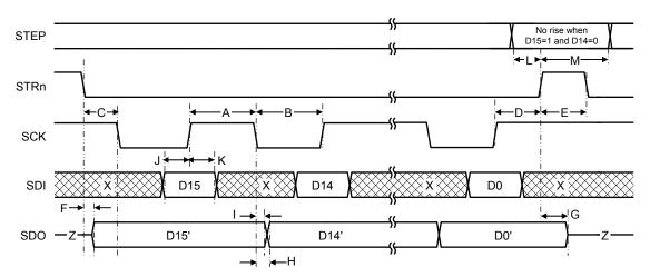
Figure 1: Serial Interface Timing Diagram
