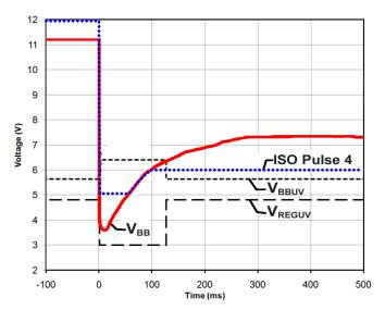
Figure 3: A4980 Response to an Undervoltage Transient
