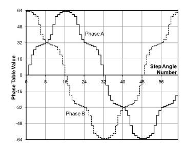
Figure 15: Resulting Example Current Profile
