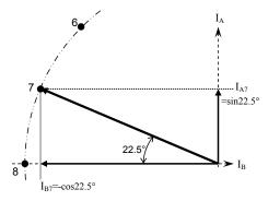
Figure A7: Calculating Phase Current Magnitudes
