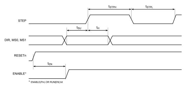
**Figure 2: Control Input Interface Timing Diagram**
