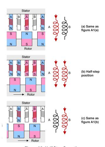
Figure A2: Half Step Operation
