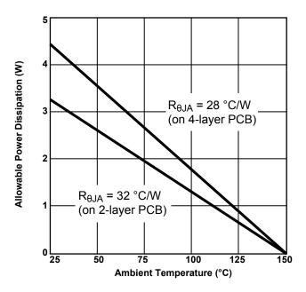
Figure 17: Allowable Power Dissipation, on Typical PCBs
