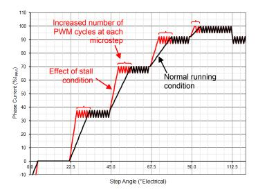
Figure 5: Effect of Stall Condition onCcurrent Rise
