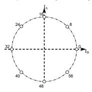
Figure 11: Half-step Phase Diagram Using STEP Input
