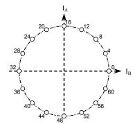
Figure 12: Quarter-step Phase Diagram Using STEP Input
