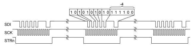
Figure 14: Serial Interface Sequence for Quarter Step in Reverse Direction
