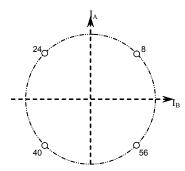
Figure 10. Full-step Phase Diagram Using STEP Input
