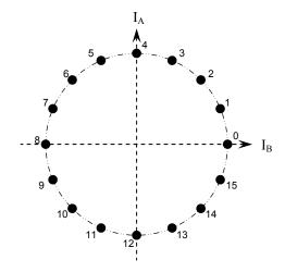
Figure A6: Phase Diagram for Quarter Step
