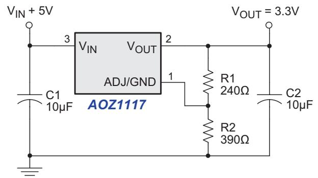
$$V_{OUT} = V_{REF} \times \left(1 + \frac{R2}{R1}\right)$$
