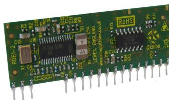
**HORNET-RX** - 433MHz 12-32V receiver with 4 relay Changeover Contacts, housed in an IP68 Enclosure.
