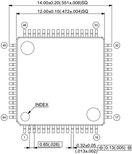
Note 1) Pins width and pins thickness include plating thickness.
