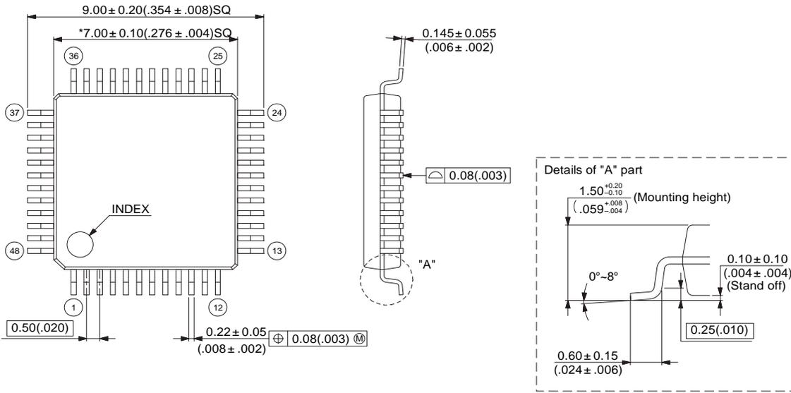
Note 1) \* : These dimensions do not include resin protrusion.
