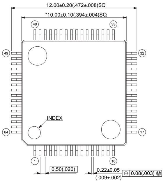
Note 1) \* : These dimensions do not include resin protrusion.
