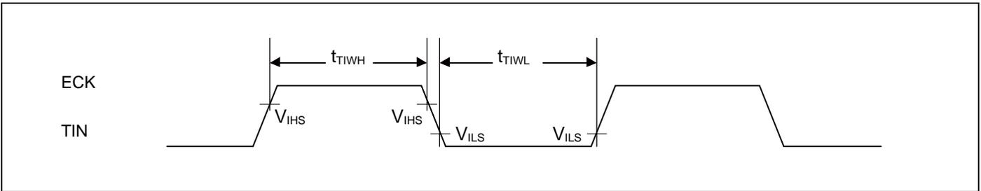
**Trigger input timing**
