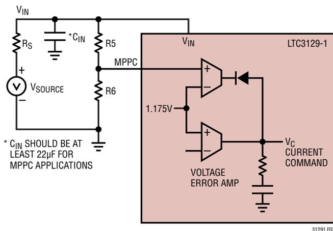
Figure 3. MPPC Amplifier with External Resistor Divider
