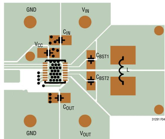
Figure 4. Typical 2-Layer PC Board Layout (MSE Package)
