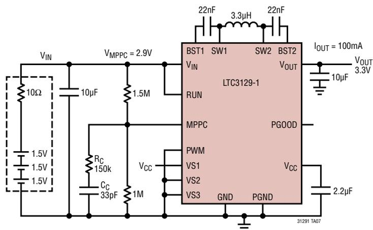
NOTE:  $R_C$  AND  $C_C$  HAVE BEEN ADDED FOR IMPROVED MPPC LOOP STABILITY WHEN USING AN INPUT CAPACITOR VALUE LESS THAN THE RECOMMENDED MINIMUM OF 22µF
