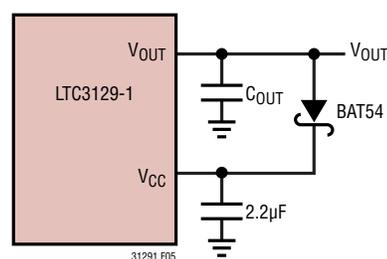
Figure 5. Example of  $V_{CC}$  Bootstrap
