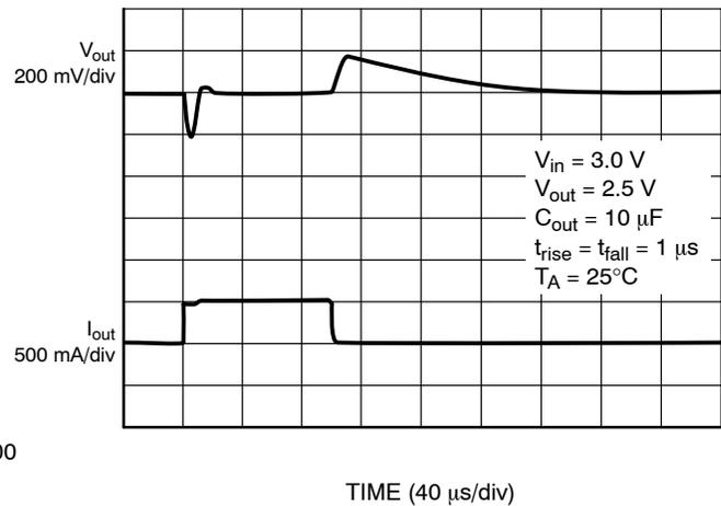
**Figure 20. Load Transient ( $V_{out} = 2.5\text{ V}$ )**
