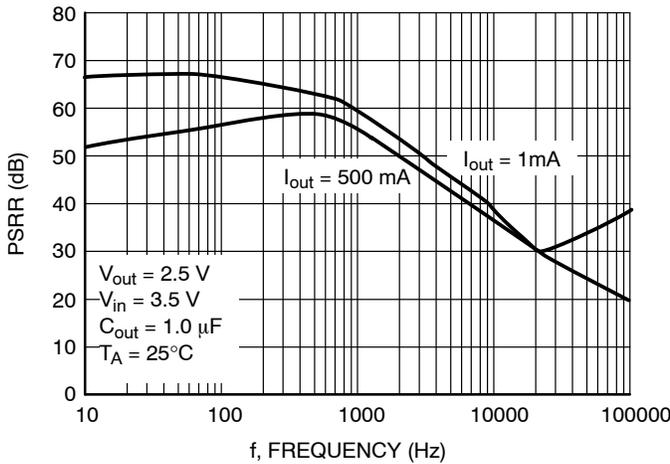
**Figure 17. PSRR vs. Frequency ( $V_{out} = 2.5\text{ V}$ )**
