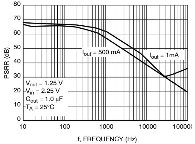
**Figure 16. PSRR vs. Frequency ( $V_{out} = 1.25\text{ V}$ )**
