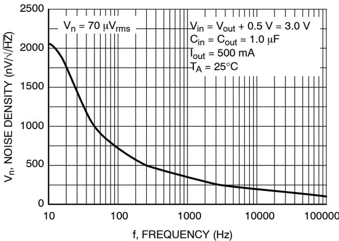
**Figure 19. Noise Density vs. Frequency ( $V_{out} = 2.5\text{ V}$ )**
