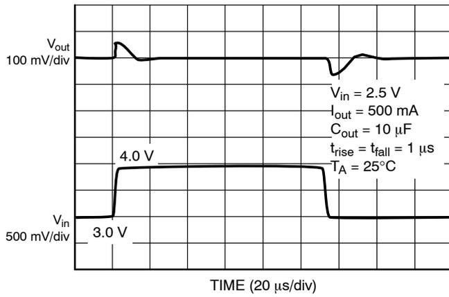
Figure 21. Line Transient ( $V_{out} = 2.5$  V)
