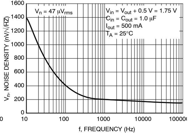
**Figure 18. Noise Density vs. Frequency ( $V_{out} = 1.25\text{ V}$ )**
