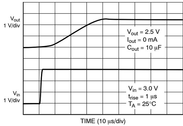
Figure 22. Startup Transient ( $V_{out} = 2.5$  V)
