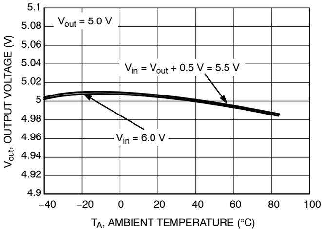
**Figure 11. Output Voltage vs. Temperature**
