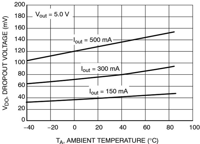
**Figure 13. Dropout Voltage vs. Temperature**
