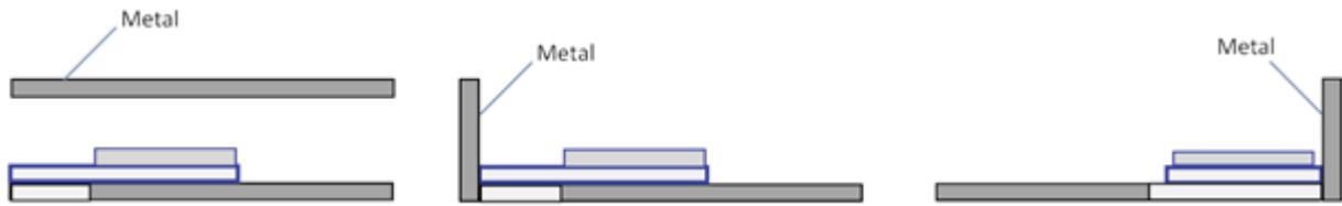
Fig 5-4. Not recommended location in Z plane
