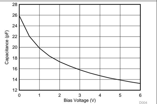
**Figure 4. Capacitance (C1 or C2) vs. Bias Voltage**
