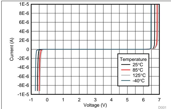
**Figure 1. DC Voltage-Current Sweep across Input, Output Pins**
