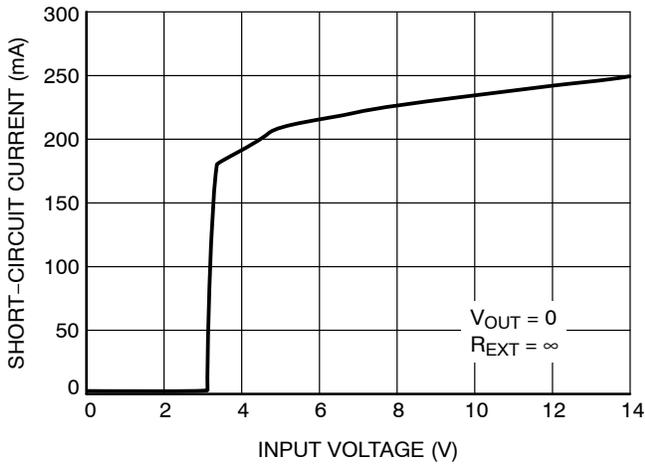
**Figure 9. Output Short-circuit Current vs. Input Voltage**
