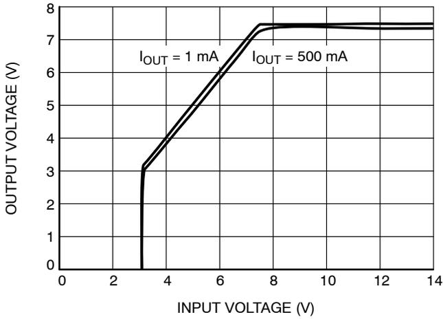
Figure 3. Dropout Characteristics
