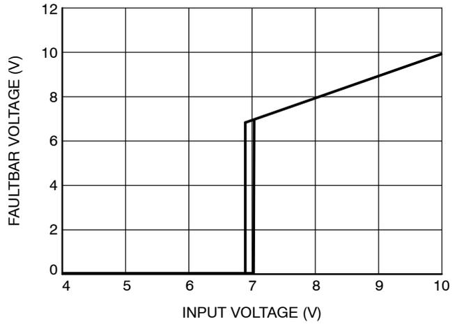
**Figure 12. Fault Bar Voltage vs. Input Voltage**
