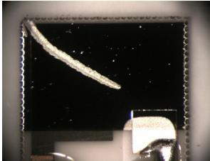
Picture 7: Sensor with contaminations
