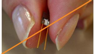
Picture 6: Sensor held with fingers without gloves on the active
