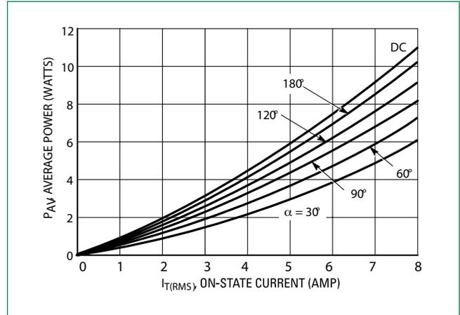
Figure 3. On-State Characteristics
