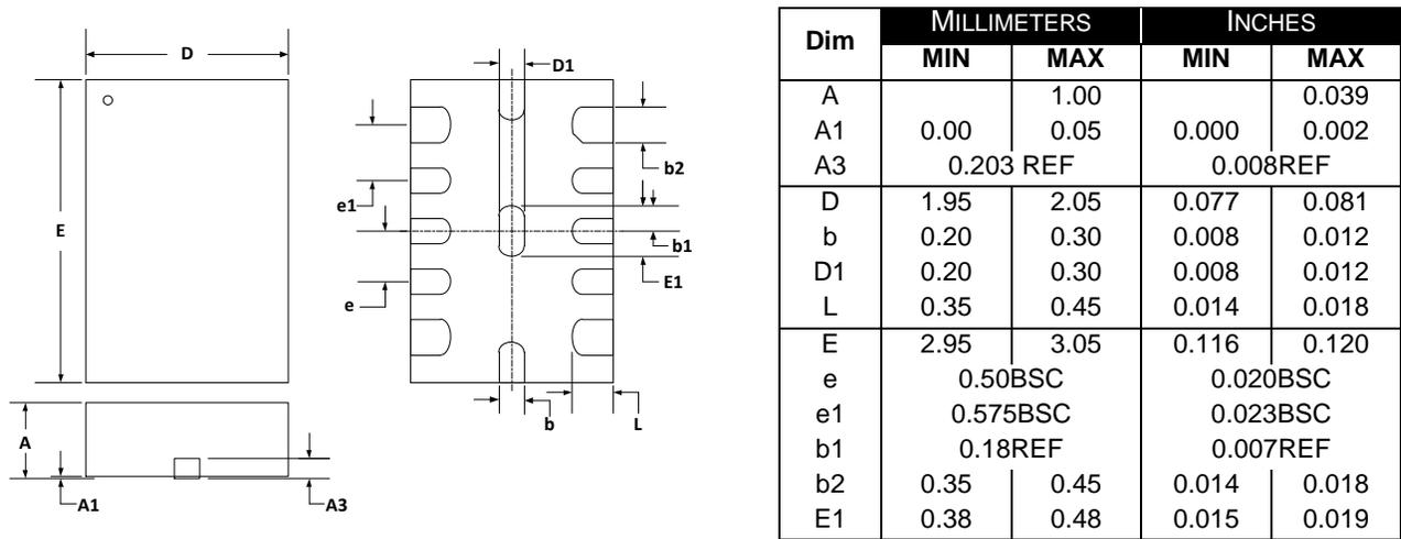
Figure 8 · LQ 12-Pin VQFN Package Dimensions
