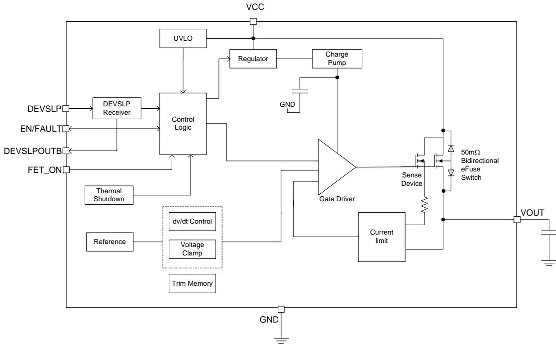
Figure 4 • Simplified Block Diagram of LX8233
