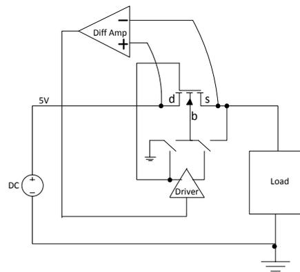
Figure 7 · Simplified reverse current detection circuitry
