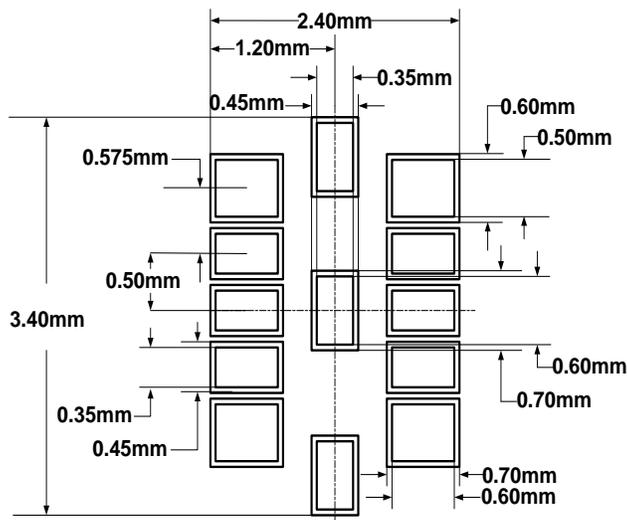
Figure 9 · LQ 12-Pin VQFN Package Land Pattern
