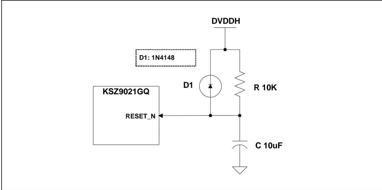
The following reset circuit is recommended for applications where reset is driven by another device (e.g., CPU or FPGA). At power-on-reset, R, C and D1 provide the necessary ramp rise time to reset the KSZ9021GQ device. The RST\_OUT\_N from CPU/FPGA provides the warm reset after power up.
