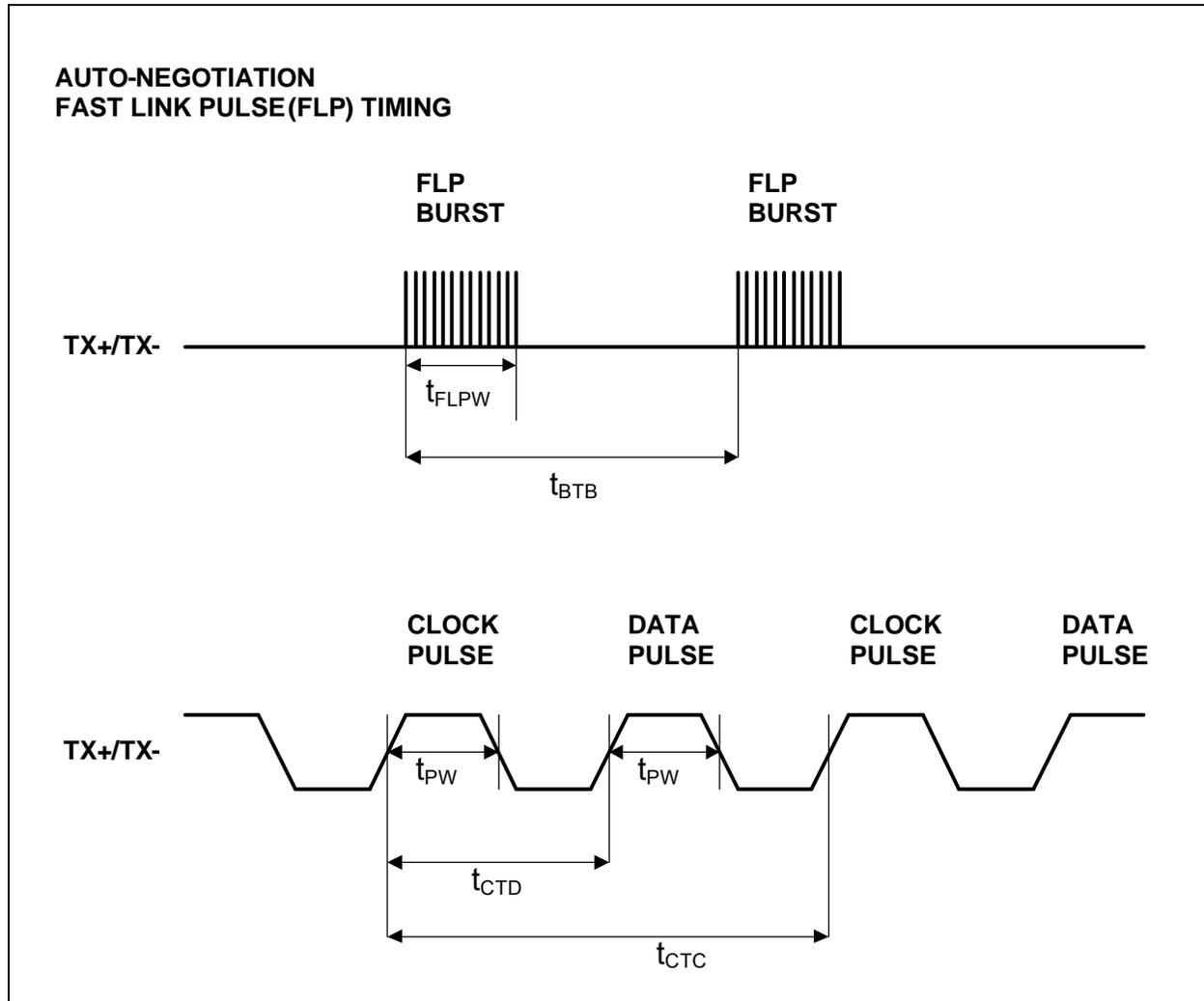
TABLE 6-5: AUTO-NEGOTIATION FAST LINK PULSE (FLP) TIMING PARAMETERS
