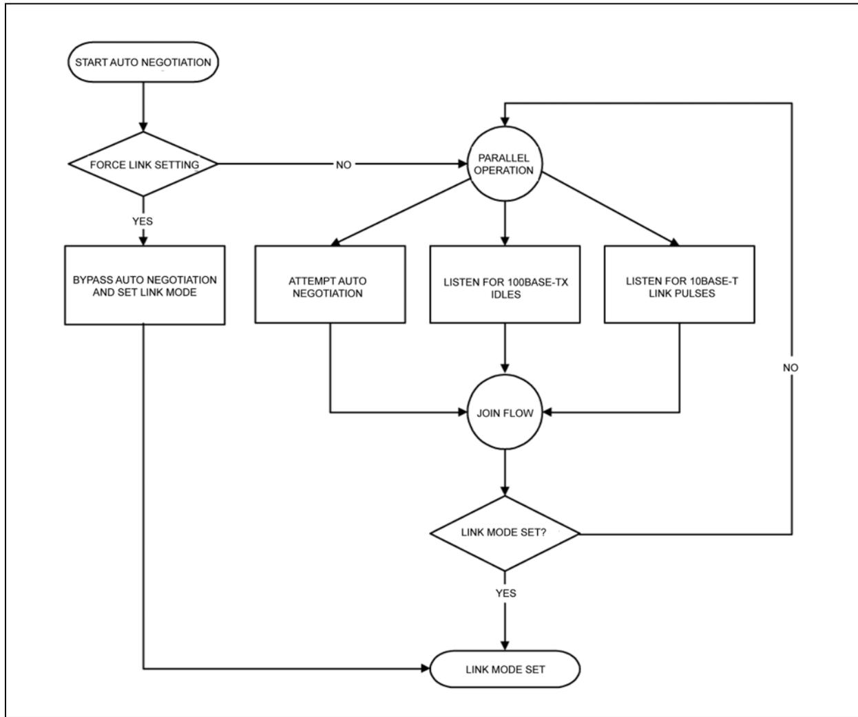
For 1000Base-T mode, auto-negotiation is required and always used to establish a link. During 1000Base-T auto-negotiation, the Master and Slave configuration is first resolved between link partners, and then the link is established with the highest common capabilities between link partners.
