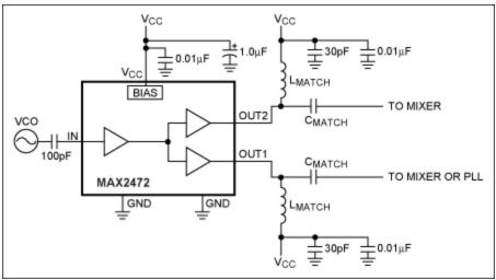
Figure 13. MAX2472 typical operating circuit.
