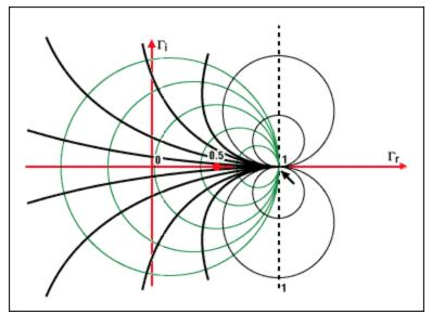
Figure 1. Fundamentals of impedance and the Smith chart.
