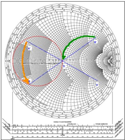
Figure 14. The network of Figure 13 with its points plotted on the Smith chart.
