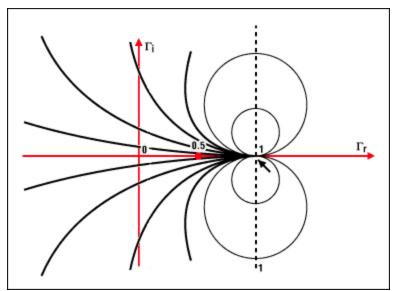
Figure 4b. The points situated on a circle are all the impedances characterized by a same imaginary impedance part value x. For example, the circle x = 1 is centered at coordinate (1, 1) and has a radius of 1. All circles (constant x) include the point (1, 0). Differing with the real part circles, x can be positive or negative. This explains the duplicate mirrored circles at the bottom side of the complex plane. All the circle centers are placed on the vertical axis, intersecting the point 1.
