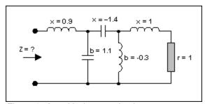
Figure 8. A multi-element circuit.
