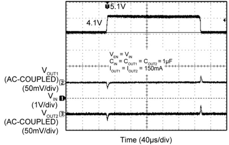
**Load Transient  $V_{OUT1}$**
