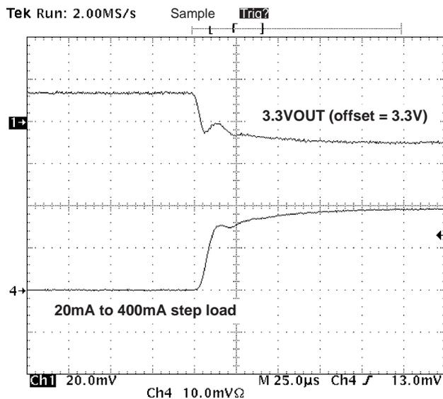
**Figure 10. 5VCC Load Transient Response Rising**
