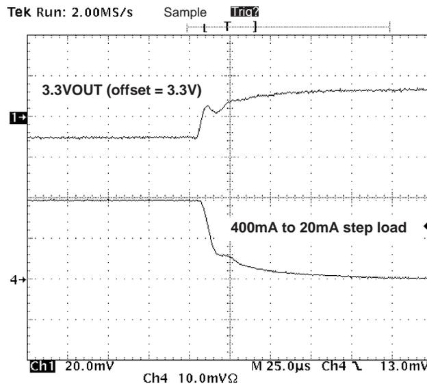
**Figure 9. 5VCC Load Transient Responses Falling**
