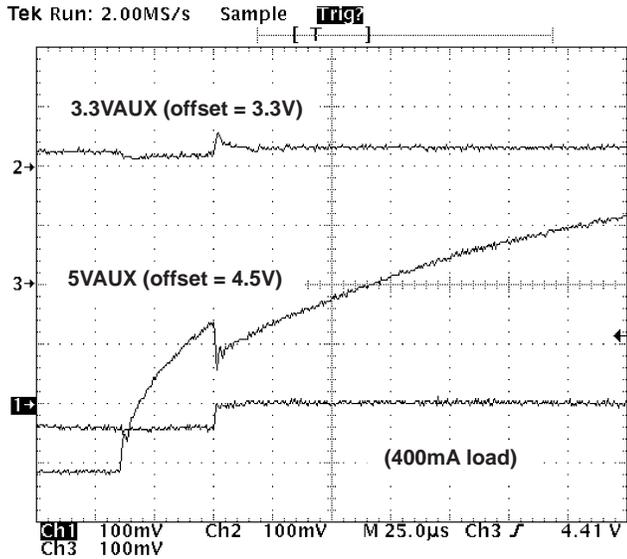
Figure 6. 5VAUX Power Up (3.3VAUX = 3.3 V)
