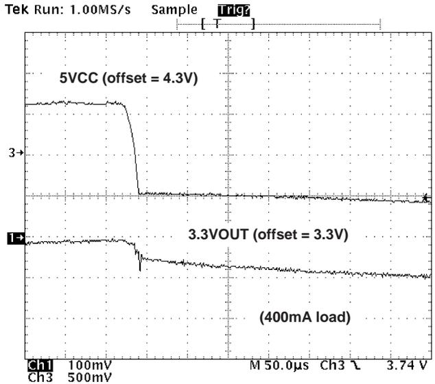
Figure 7. 5VCC Power Down (3.3VAUX = 3.3 V)
