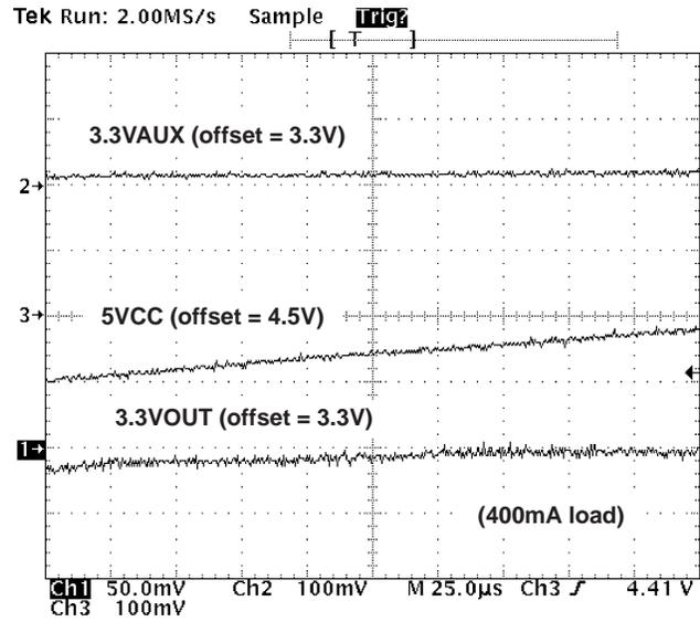
Figure 5. 5VCC Power Up (3.3VAUX = 3.3 V)
