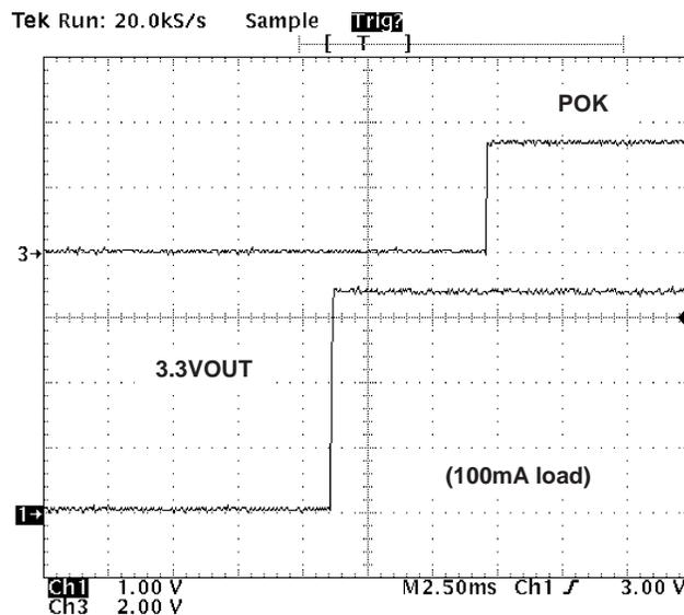
**Figure 11. 5VCC Cold Start,  $\overline{POK}$  Released**
