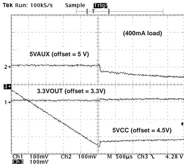
**Figure 8. 5VCC Power Down (5VAUX = 5 V)**
