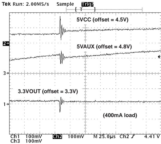
Figure 4. 5VCC Power Up (5VAUX = 5 V)
