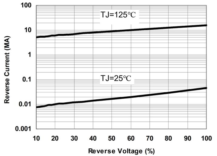
Fig.2-Typical Reverse Current
