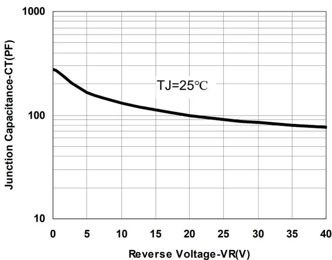
Fig.1-Typical Junction Capacitance
