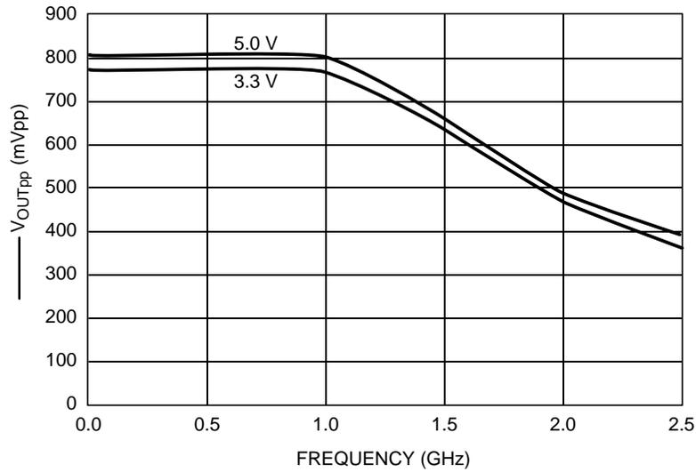
Figure 2. Typical V<sub>OUTPP</sub> (mVpp) versus Frequency (GHz) @ 25°C
