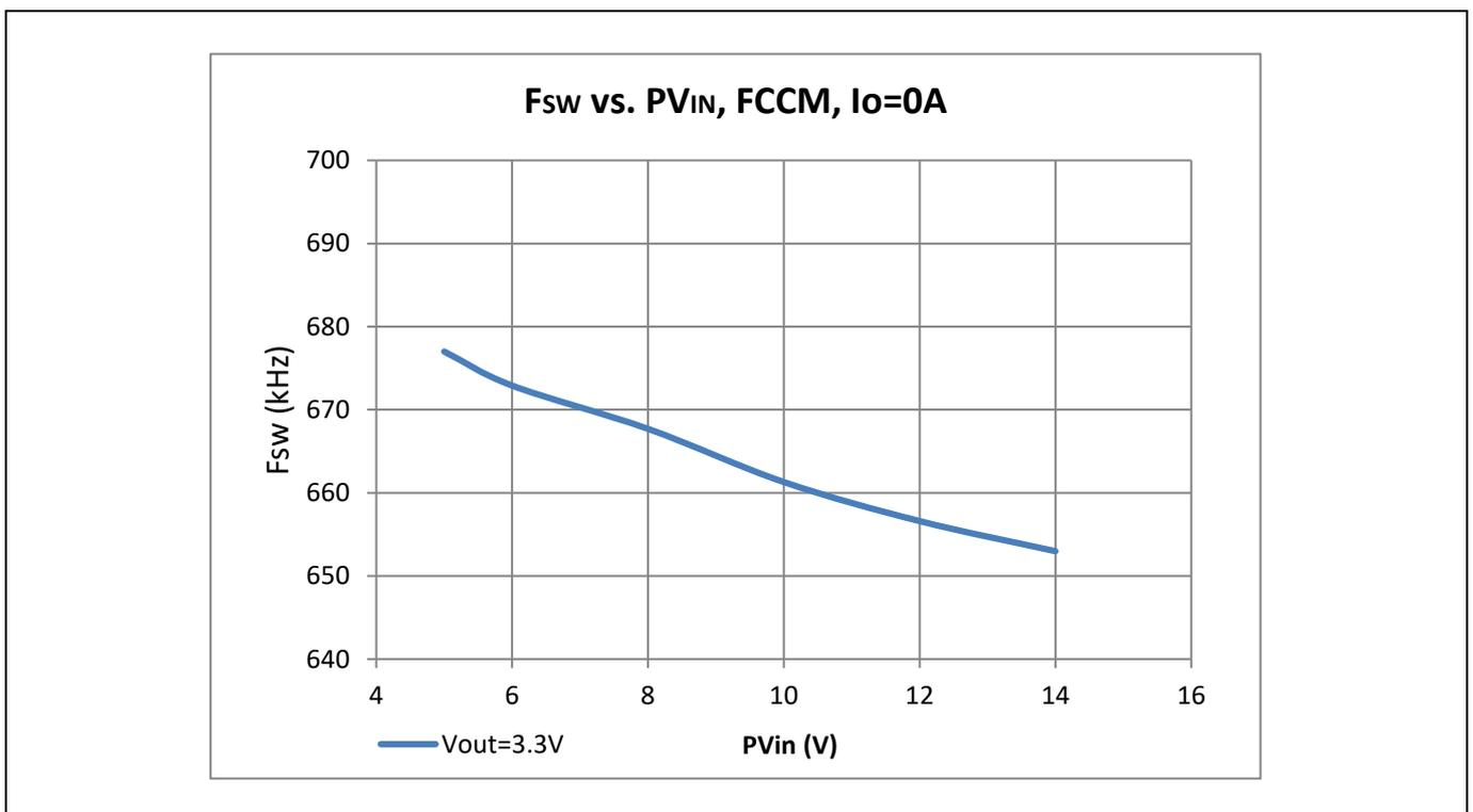
Figure 5 Switching Frequency vs. Input Voltage in FCCM, V<sub>out</sub> = 3.3 V
