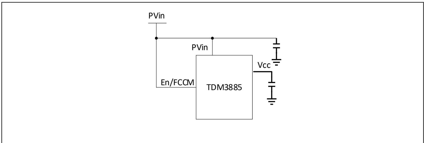
Figure 13 Single supply configuration with FCCM operation
