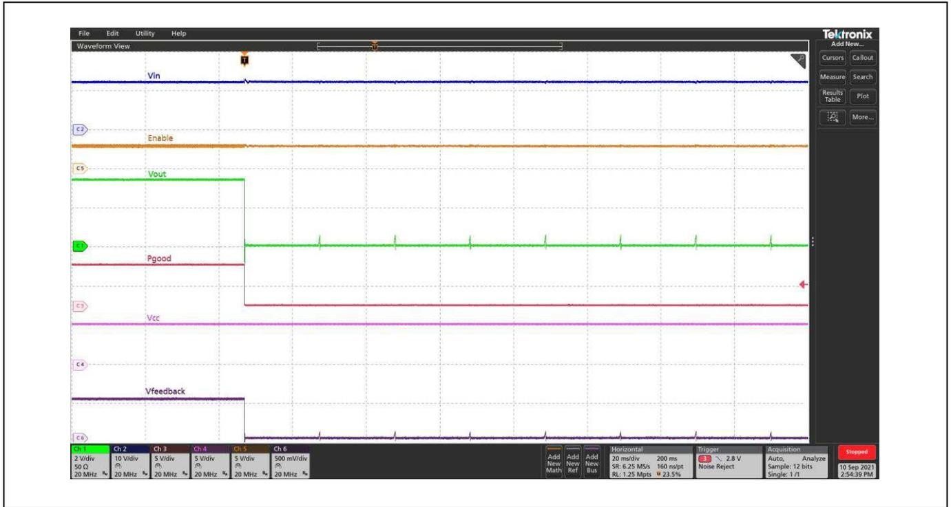
Figure 25 Short Circuit,  $P_{Vin} = 12V$ ,  $V_{out} = 3.3V$ ,  $I_{out} = 4A$ , FCCM.  $C_{H1} = V_{out}$ ,  $C_{H2} = P_{Vin}$ ,  $C_{H3} = P_{GOOD}$ ,  $C_{H4} = V_{CC}$ ,  $C_{H5} = Enable$ ,  $C_{H6} = V_{FEEDBACK}$
