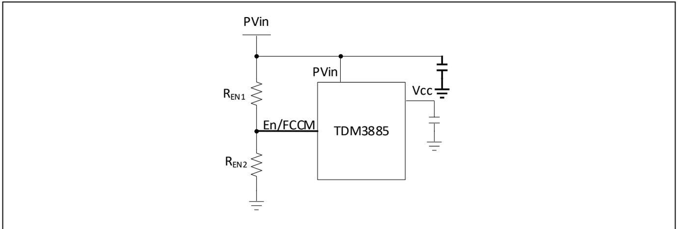
Figure 12 Single supply configuration with adjustable  $PV_{in}$  UVLO and optional FCCM or DEM
