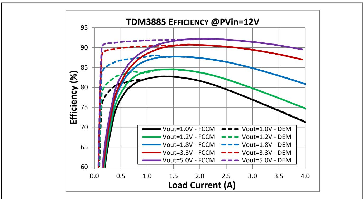
Figure 10 Efficiency Curves for  $P_{V_{in}} = 12\text{ V}$
