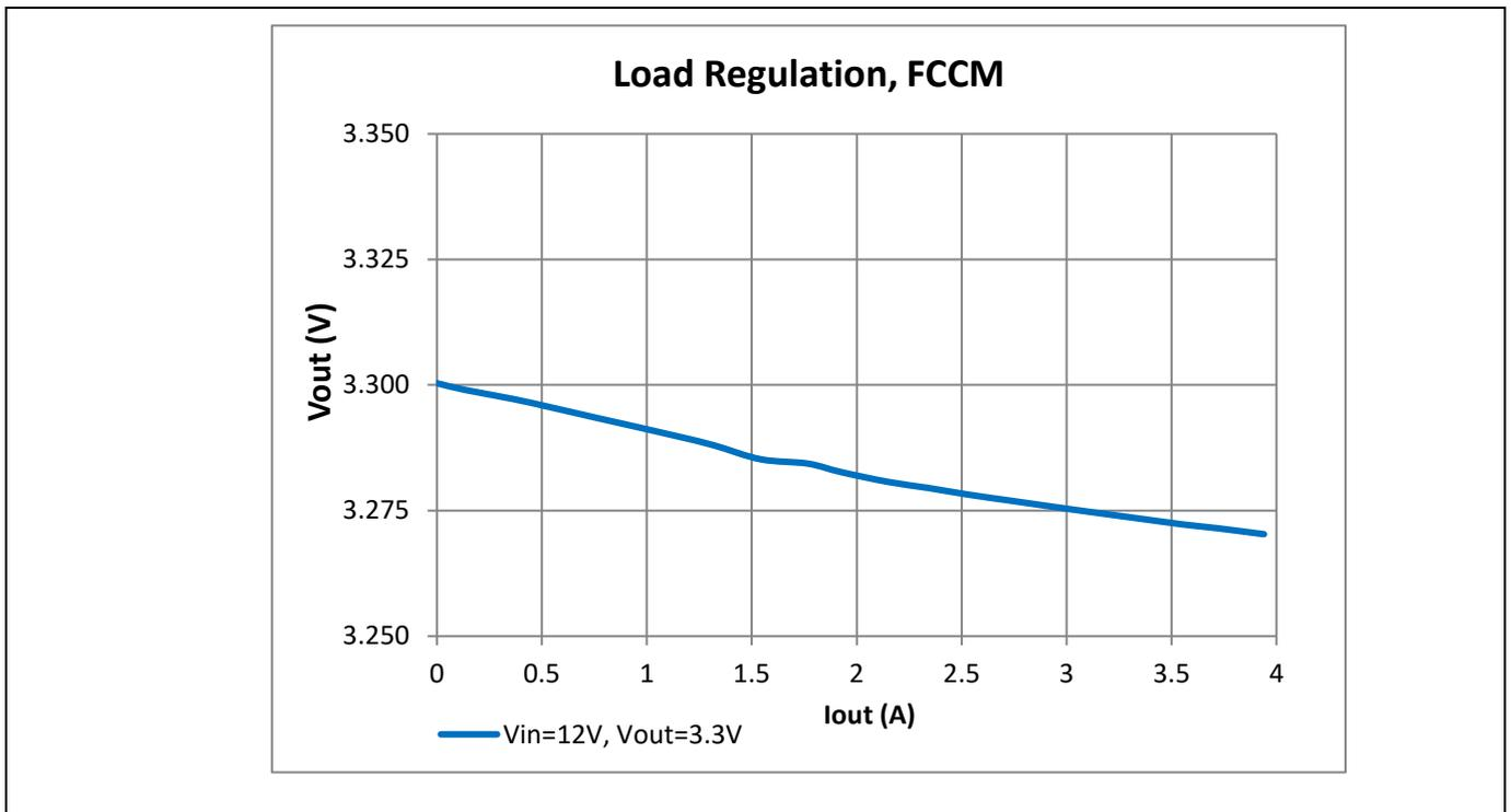
Figure 7 Load Regulation for V<sub>o</sub> = 3.3 V
