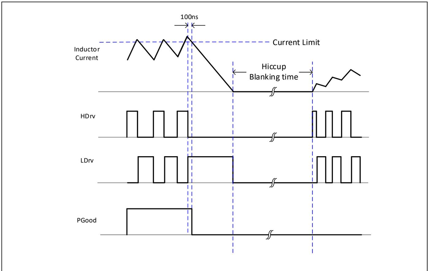
Figure 16 Illustration of OCP with hiccup Mode
