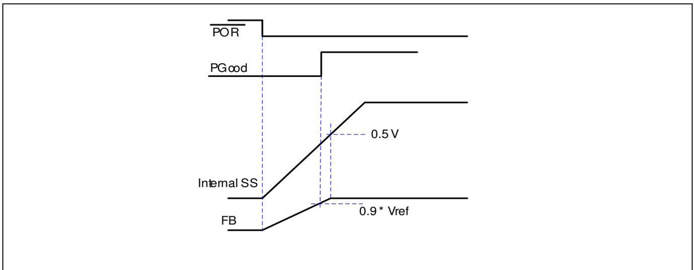
**Figure 11** Theoretical operation waveforms during soft-start
