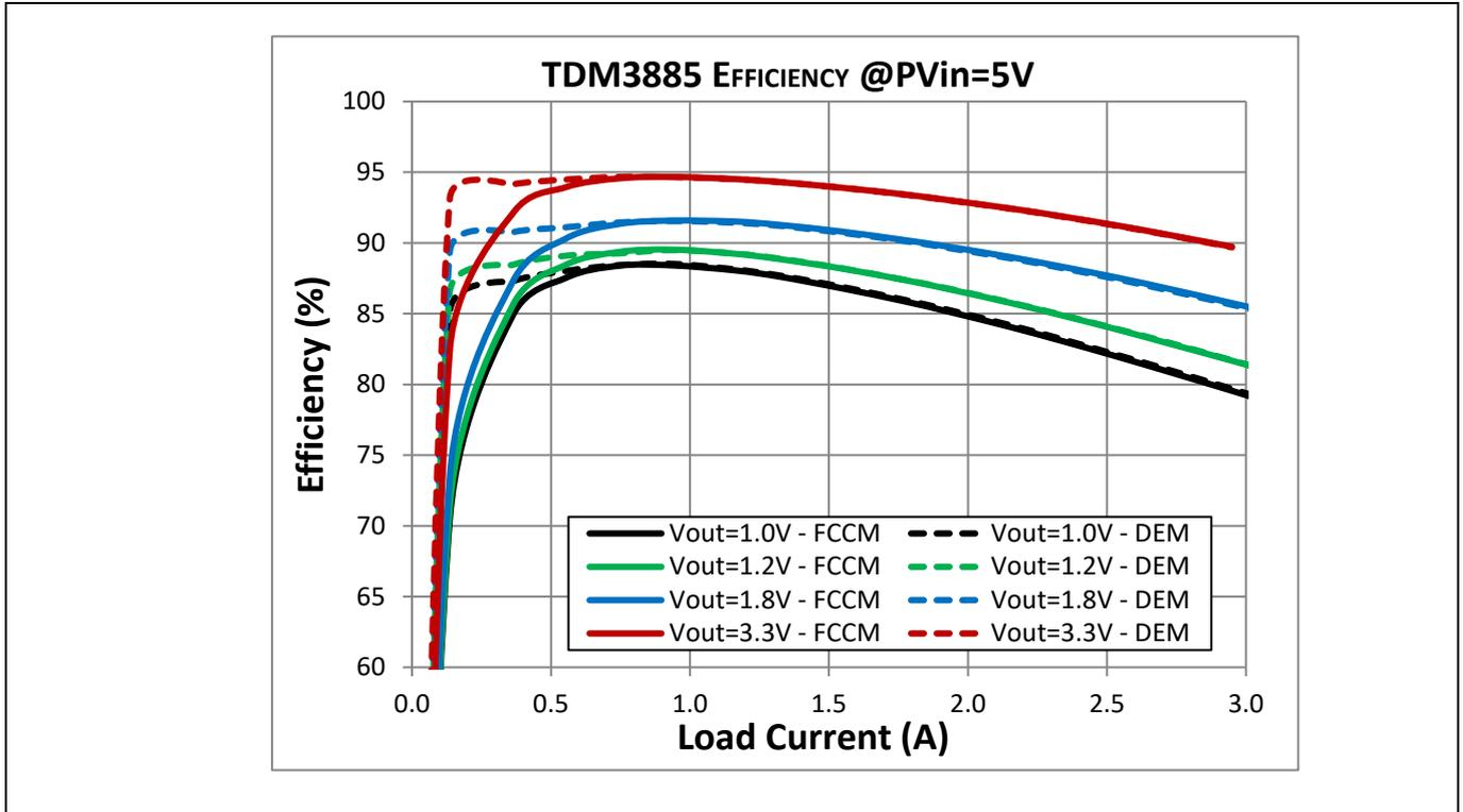
Figure 9 Efficiency Curves for  $P_{V_{in}} = 5\text{ V}$
