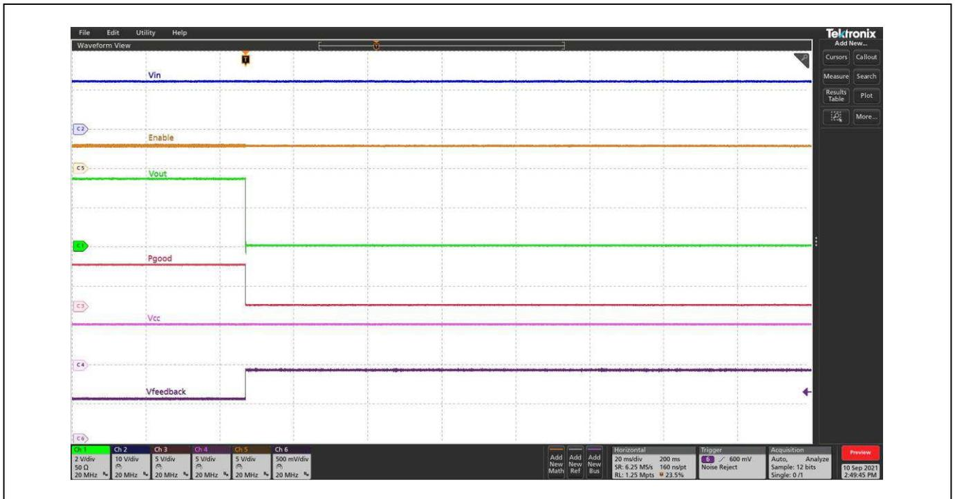
**Figure 24 OVP,  $PV_{in} = 12V$ ,  $V_{out} = 3.3V$ ,  $I_{out} = 0A$ , FCCM.  $C_{H1} = V_{out}$ ,  $C_{H2} = PV_{in}$ ,  $C_{H3} = P_{GOOD}$ ,  $C_{H4} = V_{CC}$ ,  $C_{H5} = Enable$ ,  $C_{H6} = V_{FEEDBACK}$**
