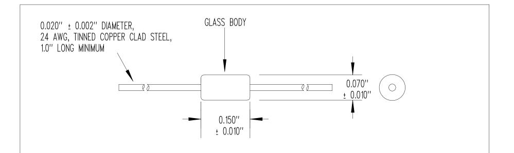
RESISTANCE @  $+25^{\circ}\text{C} = 100,000 \ \Omega \pm 5\%$  RESISTANCE/TEMPERATURE CURVE = ''R'' BEAT '' $\beta$ '' (0 TO  $+50^{\circ}\text{C}$ ) =  $4,140^{\circ}\text{K}$  NOMINAL TEMPERATURE COEFFICIENT @  $+25^{\circ}\text{C} = -4.68\%$ /°C NOMINAL DISSIPATION CONSTANT = 2 mW/°C NOMINAL THERMAL TIME CONSTANT = 5 SECONDS NOMINAL (STILL AIR) THERMAL TIME CONSTANT = 0.5 SECONDS NOMINAL (STIRRED OIL) MAXIMUM TEMPERATURE RATING =  $+300^{\circ}\text{C}$
