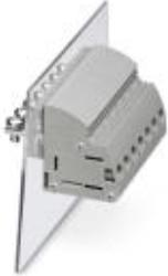
Panel feed-through terminal block, Connection method: Screw connection, Cable lug connection, Load current : 101 A, Cross section: 6 mm<sup>2</sup> - 25 mm<sup>2</sup>, AWG 10 - 4, Connection direction of the conductor to plug-in direction: 90 °, Width: 12.1 mm, Color: gray
