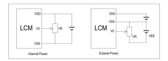
$V_{DD\sim}V_0$ : LCD Driving voltage
