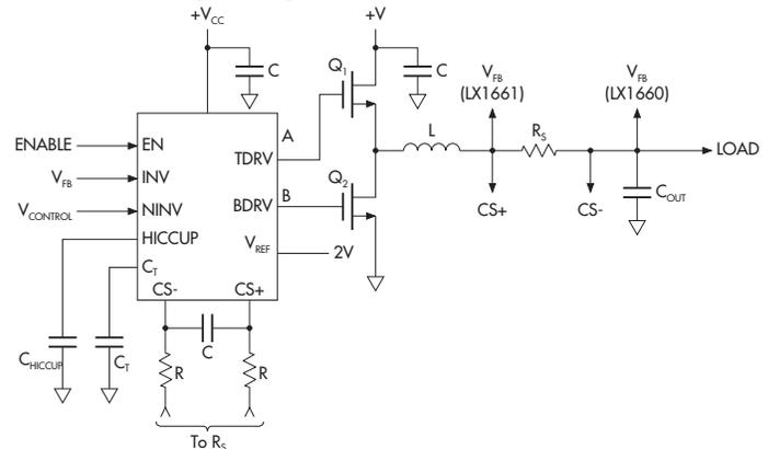
Figure 2 — LX1660 / 1661 General Circuit Configuration
