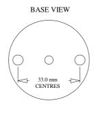
Fixing holes 2 x Ø5.5 mm, Centre hole Ø4.5 mm
