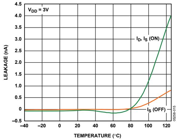
Figure 8. Leakage vs. Temperature,  $V_{DD} = 3 V$
