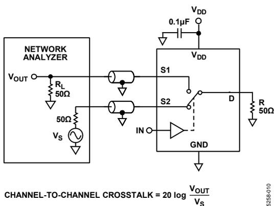
Figure 23. Channel-to-Channel Crosstalk
