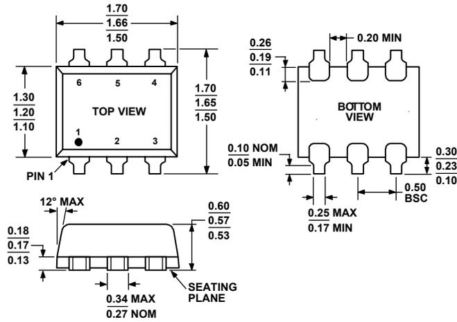
Figure 25. 6-Lead Small Outline Transistor Package [SOT-66]
