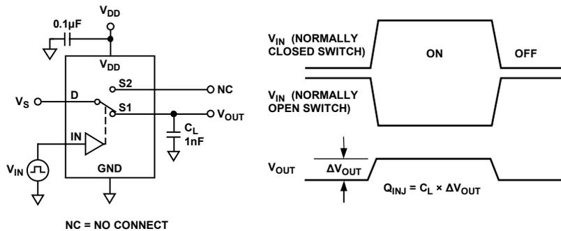
Figure 21. Charge Injection
