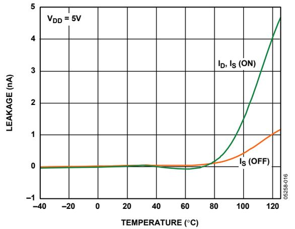
Figure 7. Leakage vs. Temperature,  $V_{DD} = 5 V$
