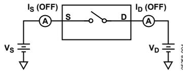
Figure 17. Off Leakage
