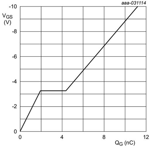
$V_{DS} = -30\text{ V}; I_D = -2.1\text{ A}; T_j = 25\text{ }^\circ\text{C}$
