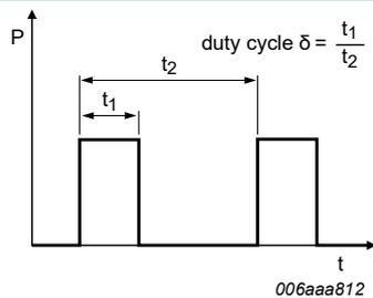
Fig. 17. Duty cycle definition
