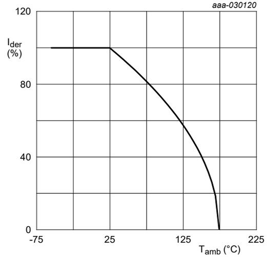
$$I_{der} = \frac{I_D}{I_{D(25^\circ\text{C})}} \times 100 \%$$
