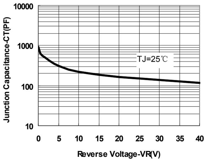
**Fig.1-Typical Junction Capacitance**
