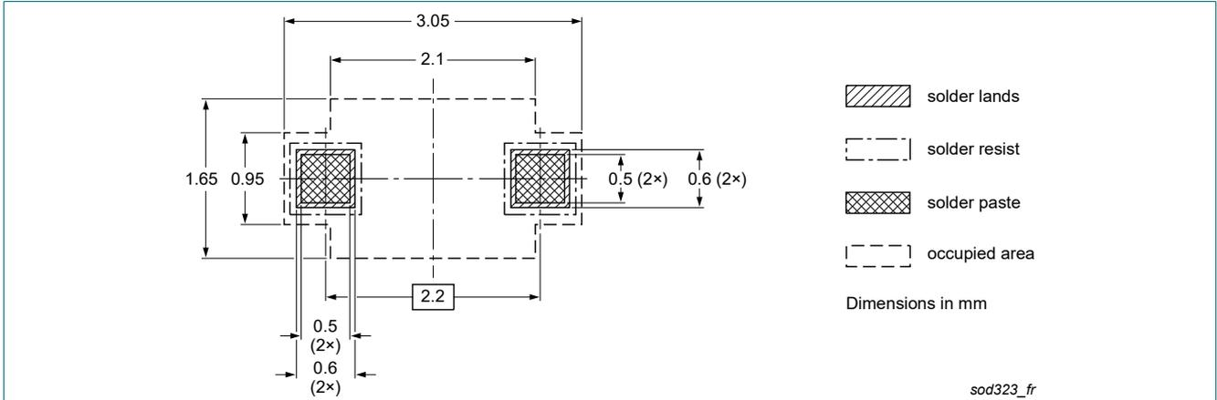
**Fig. 9. Reflow soldering footprint for SOD323**
