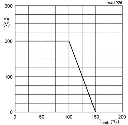
Fig. 6. Maximum permissible continuous reverse voltage as a function of the ambient temperature
