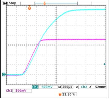
Figure 3. This scope photo illustrates the tracking of  $V_{I/O}$  (upper trace) and  $V_{CORE}$  in the circuit of Figure 2, where  $V_{I/O} = 3.3V$ ,  $V_{CORE} = 1.8V$ , and both loads are adjusted to 1A.
