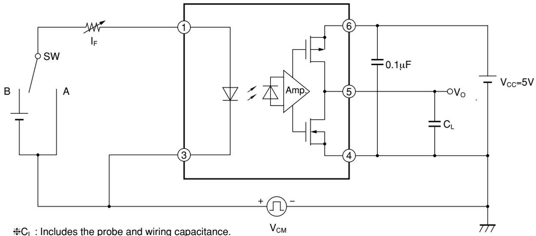
\* $C_L$  : Includes the probe and wiring capacitance.
