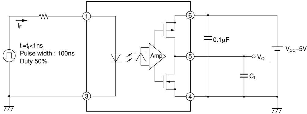
\* $C_L$  : Includes the probe and wiring capacitance.
