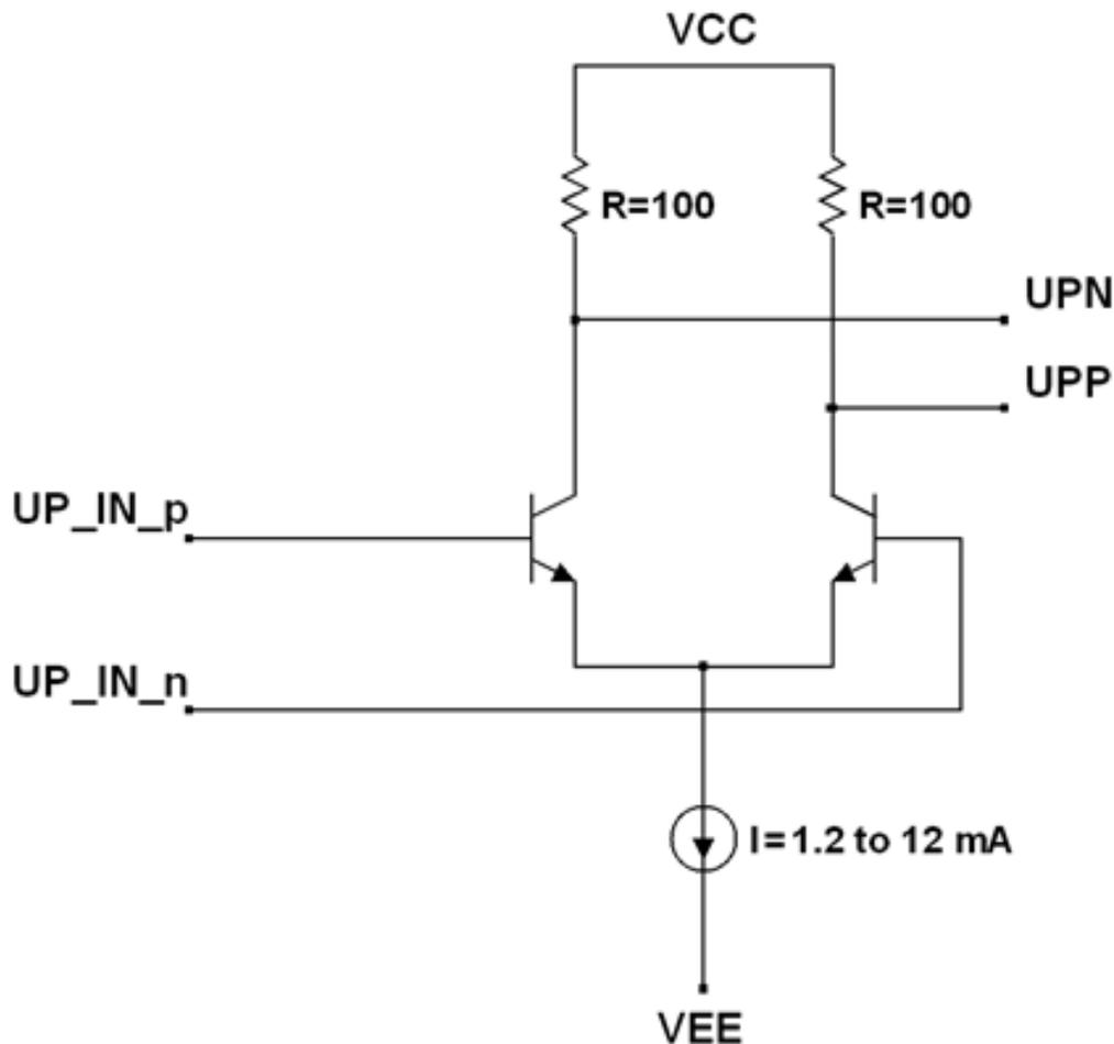
*Simplified Charge Pump Output Circuit*
