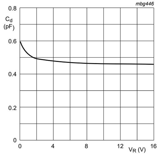
$f = 1\text{ MHz}; T_{amb} = 25\text{ }^{\circ}\text{C}$
