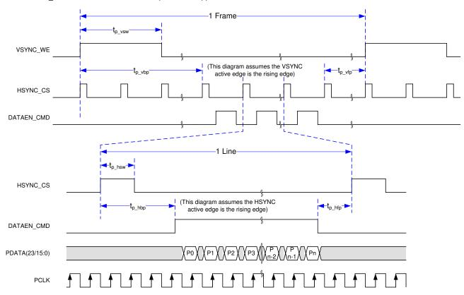
Figure 6-7. Parallel Interface Frame Timing
