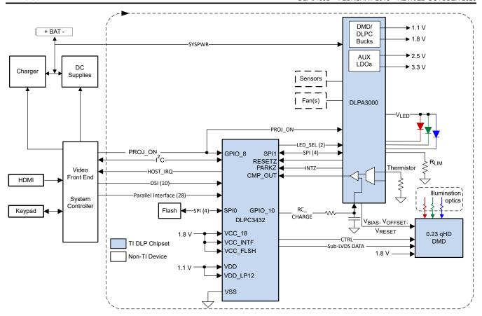
Figure 8-2. Typical Simplified Application Schematic (using DLPA3000)
