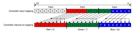
Figure 7-4. RGB-565 and YCbCr-565 I/O Mapping
