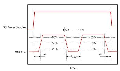
Figure 6-6. Power-Up and Power-Down RESETZ Timing
