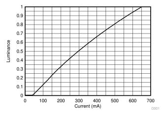
Figure 8-3. Typical Luminance vs Current
