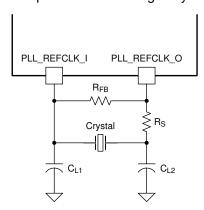
$$\begin{split} &C_L = \text{Crystal load capacitance (farads)} \\ &C_{L1} = 2 \times (C_L - \text{Cstray\_pll\_refclk\_i}) \\ &C_{L2} = 2 \times (C_L - \text{Cstray\_pll\_refclk\_o}) \\ &\text{where:} \end{split}$$
