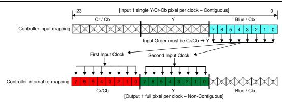
Figure 7-7. 8-Bit Serial YCbCr-422 I/O Mapping
