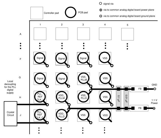
Figure 10-1. PLL Filter Layout
