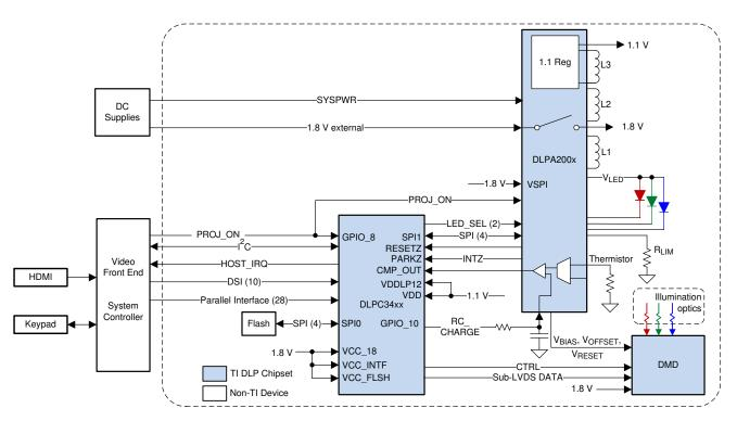
Figure 8-1. Typical Simplified Application Schematic (using DLPA200x)
