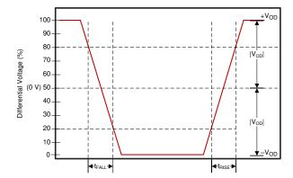
V<sub>CM</sub> is removed when the signals are viewed differentially.
