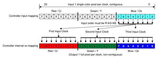
Figure 7-6. 8-Bit RGB-888 or YCbCr-888 I/O Mapping
