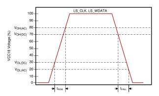
Figure 6-3. LS\_CLK and LS\_WDATA Slew Rate
