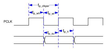
Figure 6-8. Parallel Interface Pixel Timing
