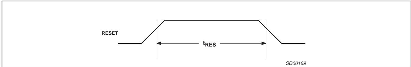
Figure 10. Reset Timing
