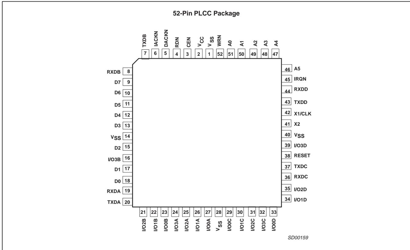
Figure 1. Pin configuration
