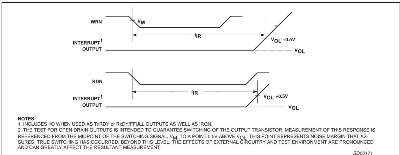
Figure 12. Interrupt Timing
