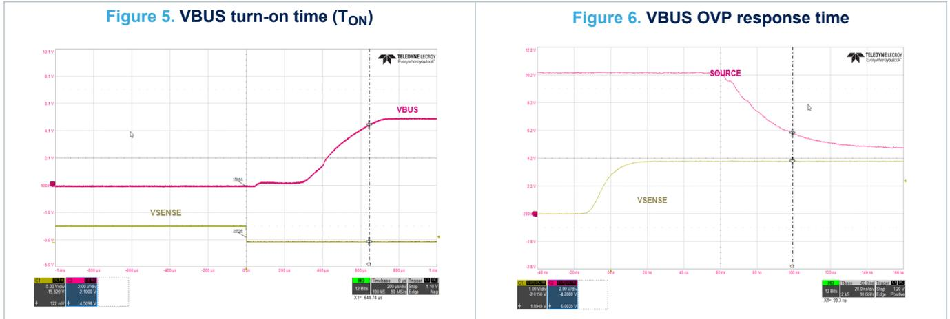
Note: Test conditions for Figure 5 and Figure 6: TCPP03-M20 is in hibernate mode  $VCC\_VCONN = ENABLE = 0 V$ ,  $VBUS = 5 V$ .
