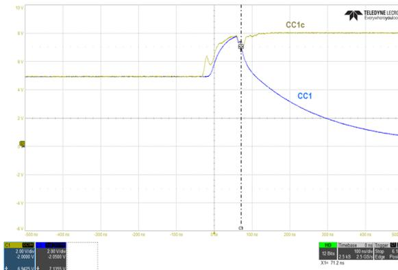
Note: Test conditions for Figure 7: TCPP03-M20 in normal mode  $VCC\_VCONN = +5 V$ ,  $ENABLE = 3.3 V$ ,  $VBUS = 0 V$ .
