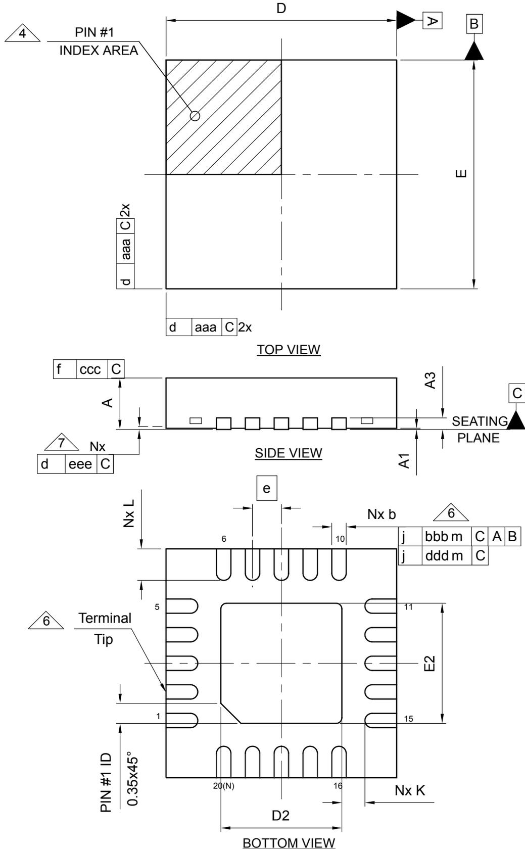
**Table 24. QFN-20L 4.0 x 4.0 x 0.75 mm package mechanical data**
