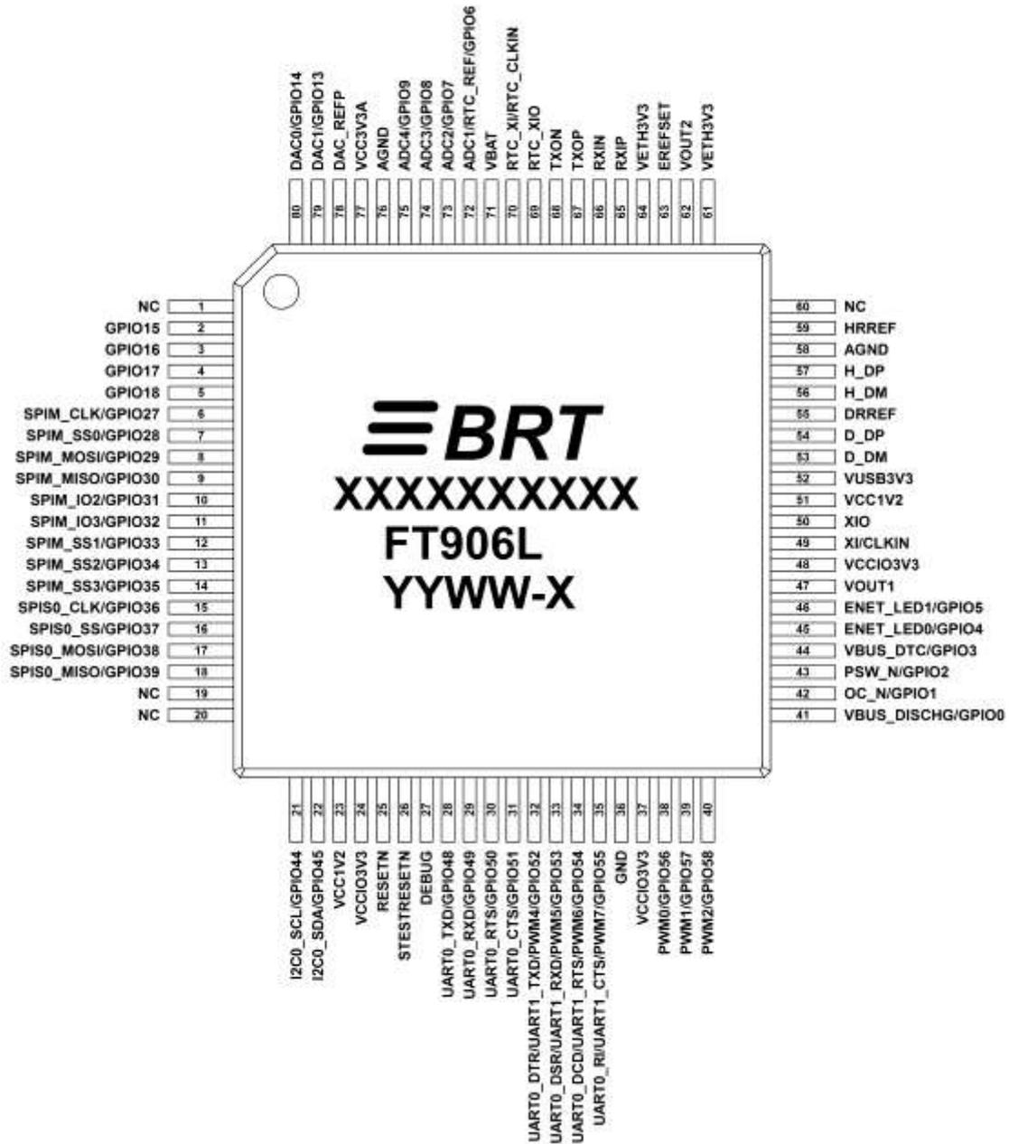
Figure 3-6 - Pin Configuration FT906L (top-down view)
