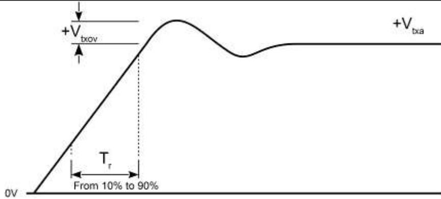
Figure 5-4 - 100Base-TX Transmission Waveform
