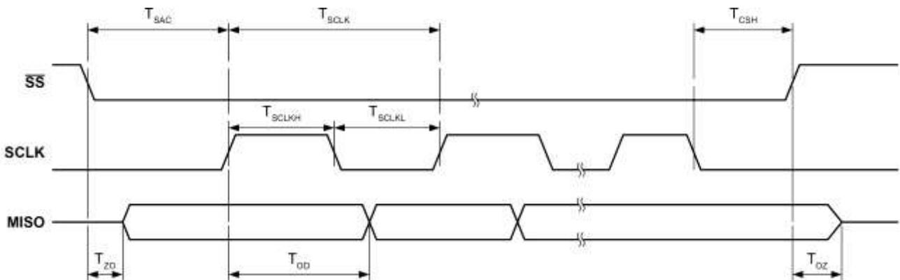
**Figure 5-8 - Definition of SPI Slave Timing Mode 0**
