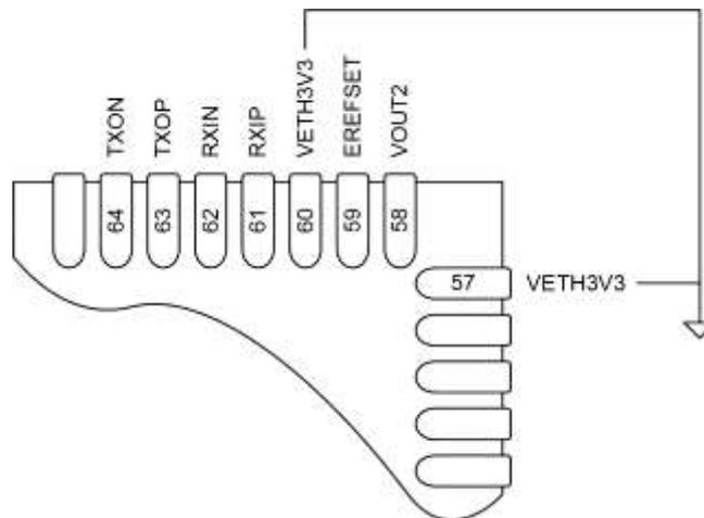
**Figure 6-8 - Unused Ethernet Connection (QFN)**
