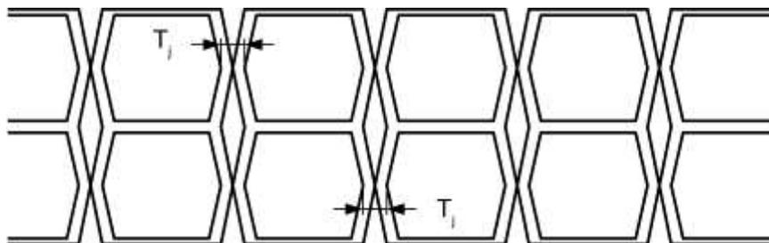
**Figure 5-3 - 100Base-TX Jitter Timing**
