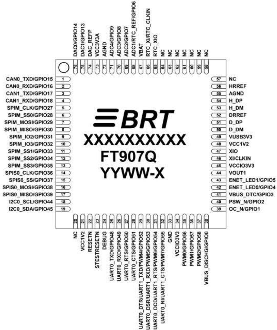
Figure 3-3 - Pin Configuration FT907Q (top-down view)
