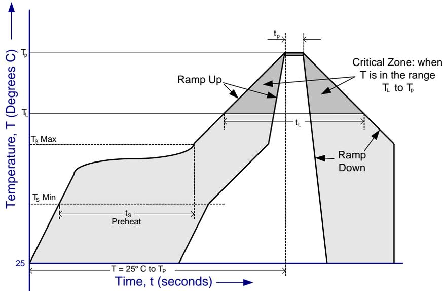
**Figure 7-5 - FT905 Solder Reflow Profile**
