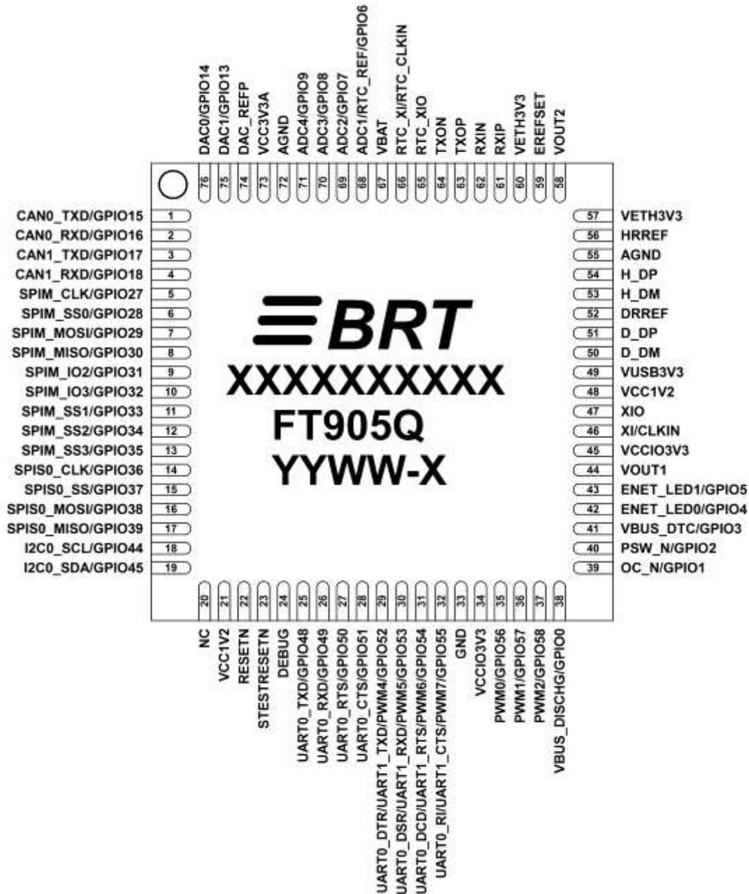
Figure 3-1 - Pin Configuration FT905Q (top-down view)
