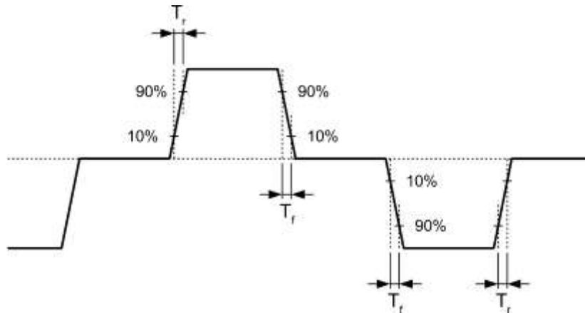
**Figure 5-2 - 100Base-TX  $T_{r/f}$  Timing**
