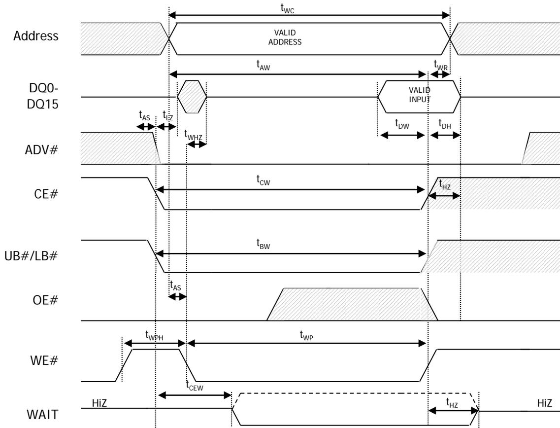
**Figure 35: Four-Word Burst WRITE Operation – Variable Latency**
