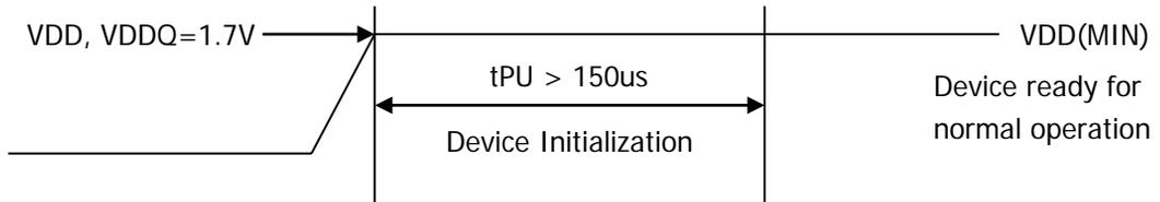
**Figure 19: DPD Entry and Exit Timing Parameters**
