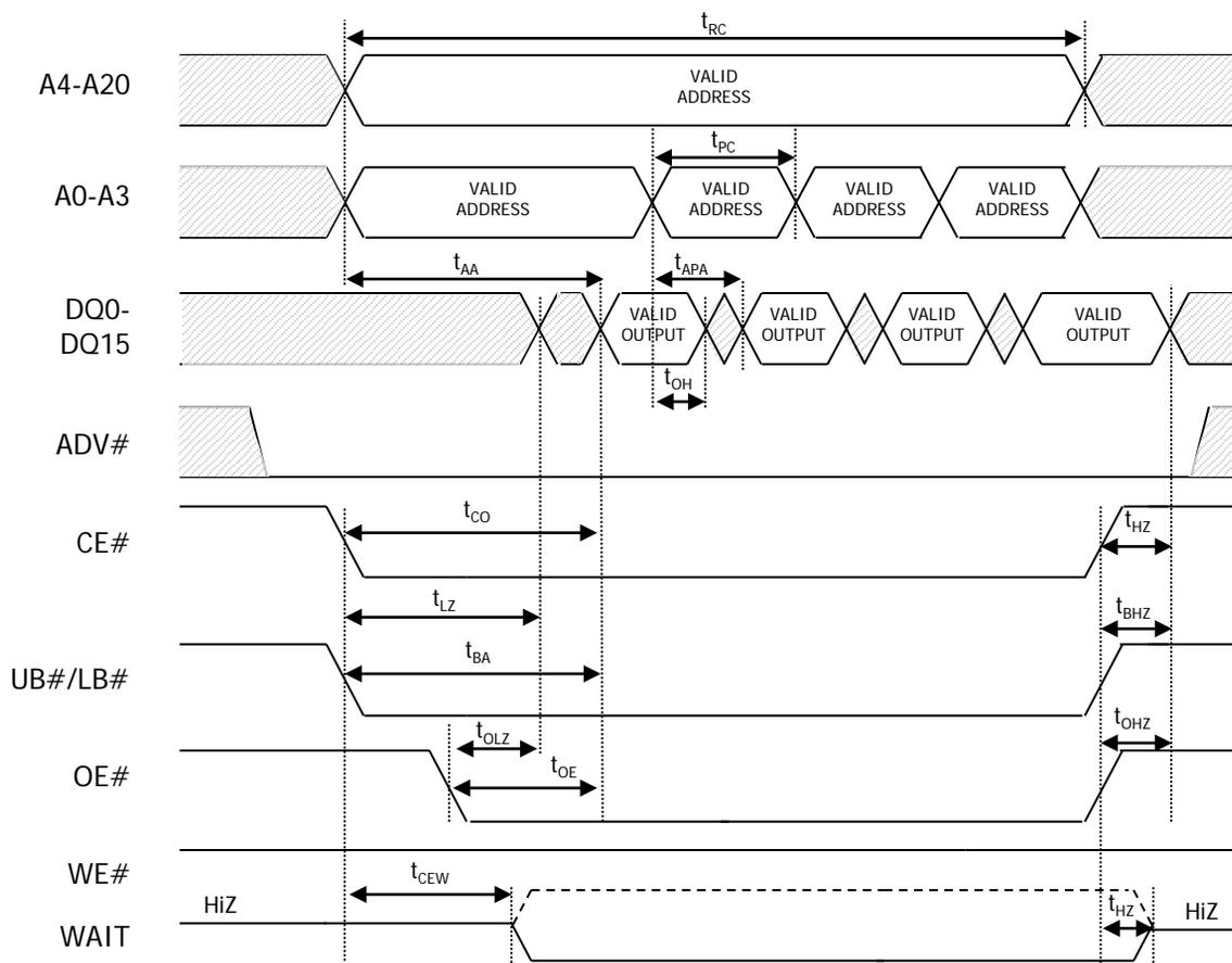
Figure 23: CLK Timings for Burst Operations
