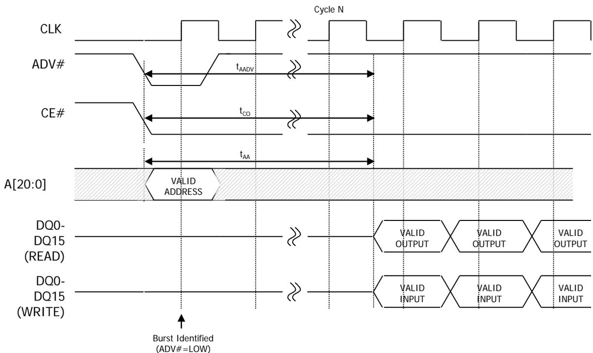
**Operating Mode (BCR[15]) Default = Synchronous Operation**
