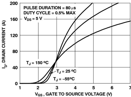
Figure 5. Transfer Characteristics
