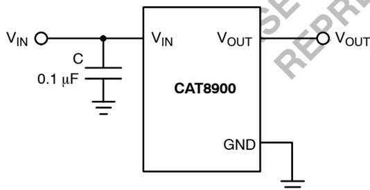
Figure 1. Application Circuit
