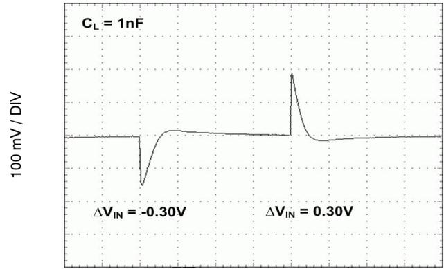
Figure 9. Line Transient Response with Capacitive Load
