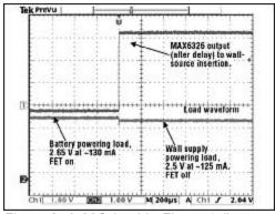
Figure 2. A  $20\Omega$  load in Figure 1 (bottom trace) registers a slight mismatch as the wall supply takes over from the battery, indicated by the change in U1's output (top trace).
