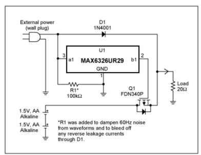
Figure 1. This circuit provides battery/wall-source switchover while debouncing the wall-source output. The low  $R_{DS(ON)}$  of Q1 reduces its voltage drop to less than 0.1V.
