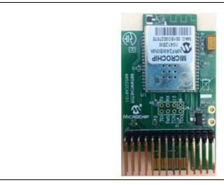
When inserting the PICtail into the development board, orient the PICtail with the module facing the microcontroller.
