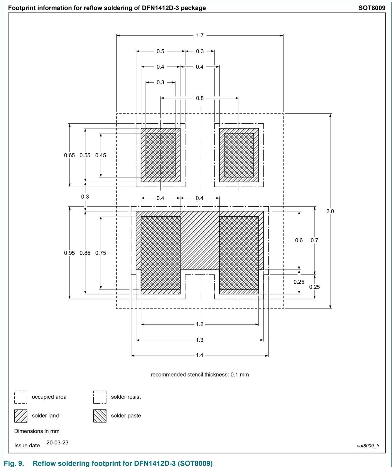
**Fig. 9. Reflow soldering footprint for DFN1412D-3 (SOT8009)**
