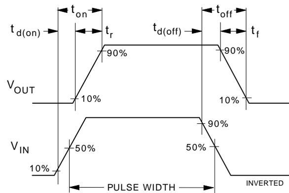
Figure 12. Switching Waveforms
