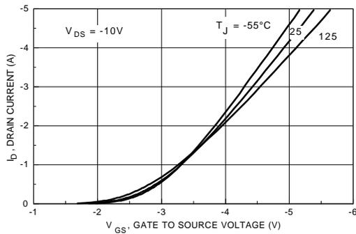
Figure 5. Transfer Characteristics
