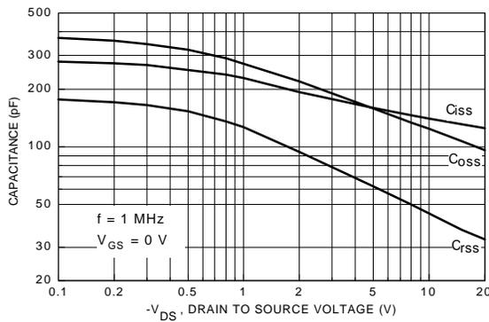
Figure 9. Capacitance Characteristics
