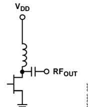
Figure 6. V<sub>DD</sub> and R<sub>FOUT</sub> Interface Schematic
