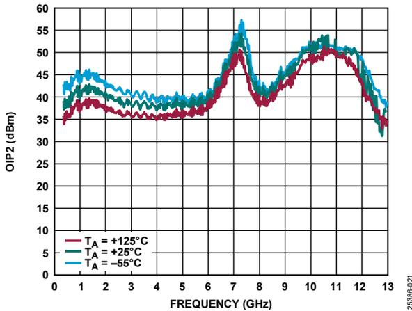
Figure 21. OIP<sub>2</sub> vs. Frequency for Various Temperatures, 300 MHz to 13 GHz, V<sub>DD</sub> = 5 V, I<sub>DQ</sub> = 60 mA, R<sub>BIAS</sub> = 1.47 kΩ, P<sub>OUT per Tone</sub> = 0 dBm
