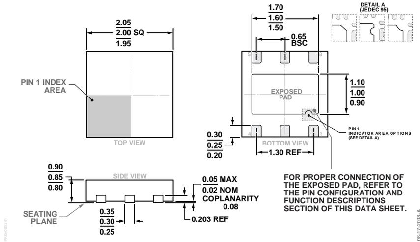
Figure 23. 6-Lead Lead Frame Chip Scale Package [LFCSP]
