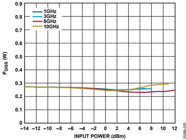
Figure 20. P<sub>DISS</sub> vs. Input Power at T<sub>A</sub> = 125°C, V<sub>DD</sub> = 5 V, I<sub>DQ</sub> = 60 mA, R<sub>BIAS</sub> = 1.47 kΩ
