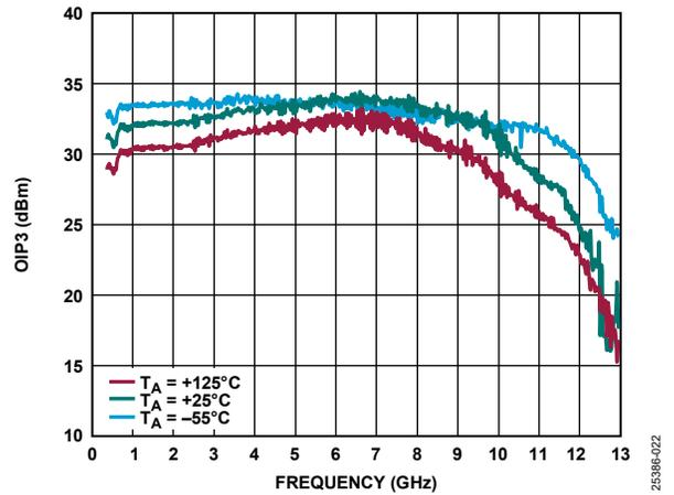
Figure 22. OIP<sub>3</sub> vs. Frequency for Various Temperatures, 300 MHz to 13 GHz, V<sub>DD</sub> = 5 V, I<sub>DQ</sub> = 60 mA, R<sub>BIAS</sub> = 1.47 kΩ, P<sub>OUT per Tone</sub> = 0 dBm
