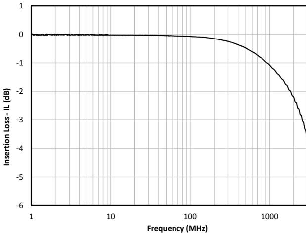
**Insertion Loss (I/O Pin to I/O Pin)**
